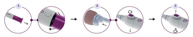
Pull the Piston to generate the vacuum and rotate to lock it.
