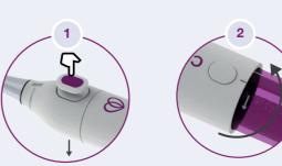
Press down on the solid-shaped side of the Button.
